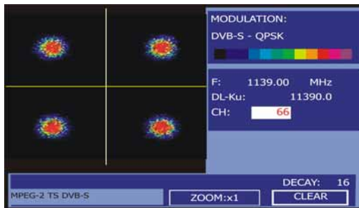
Figure 49.- Constellation Diagram. DVB-S (QPSK) signal.
