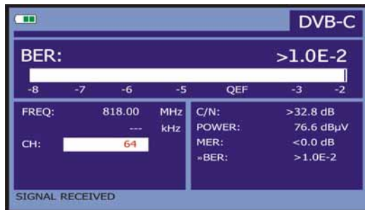
Figure 30.- DVB-C (QAM) signals BER measurement screen.
