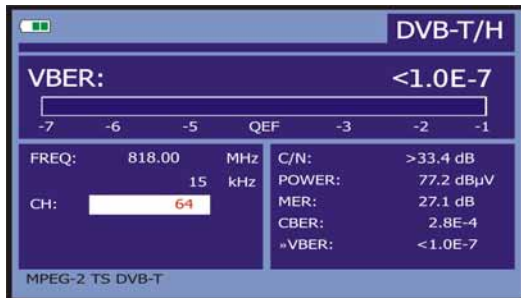
Figure 34.- DVB-T/H (COFDM) signals VBER measurement screen.
