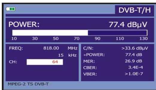
Figure 29.- Digital channel power measurement.
