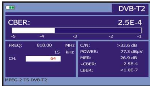
Figure 35.- CBER measurement for COFDM modulated signals.
