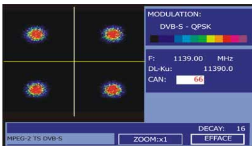
Figure 49.- Diagramme de constellation. Signal DVB-S (QPSK).
