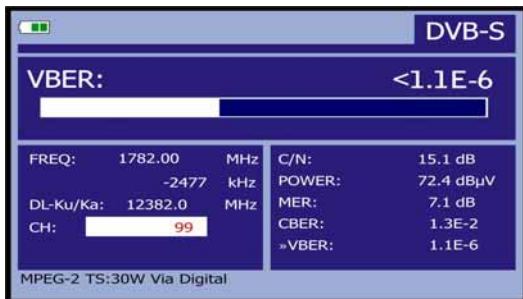
Figure 40.- DVB-S (QPSK) signals VBER measurement screen.
