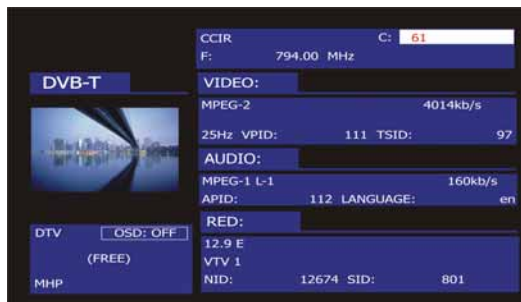
Figure 70.- Digital channel monitoring.
