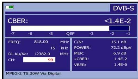
Figure 38.- DVB-S (QPSK) signals CBER measurement screen.
