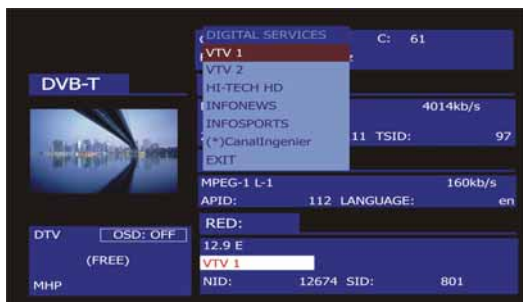
Figure 71.- Digital channel monitoring. Digital services.
