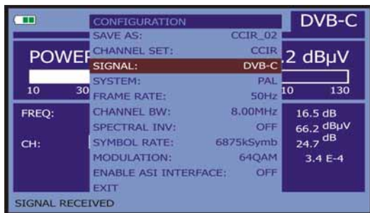
Figure 19.- Screen of measurement configuration (QAM signals).
