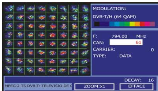
Figure 45.- Diagramme de constellation. Signal DVB-T/H (QAM 64).
