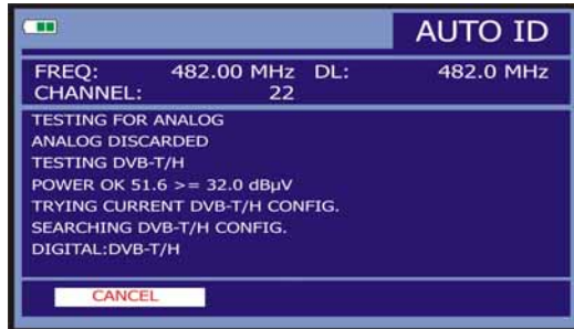
Figura 58.- Automatic identification of the signal.
