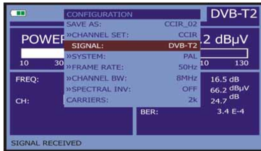
Figure 21.- Screen of measurement configuration (COFDM signals).
