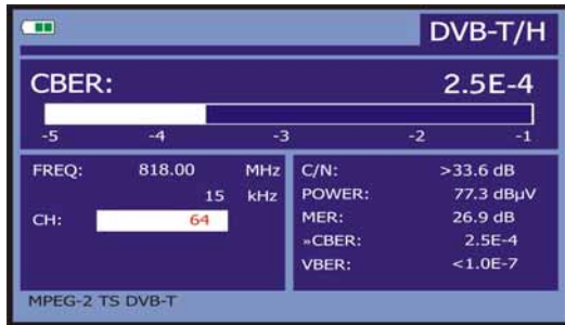
Figure 32.- DVB-T/H (COFDM) signals CBER measurement screen.
