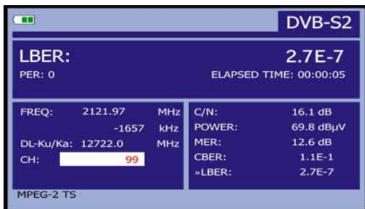
Figure 42.- DVB-S2 (QPSK/8PSK) signals LBER measurement screen.
