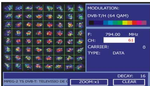
Figure 45.- Constellation Diagram. DVB-T/H (64 QAM) signal.
