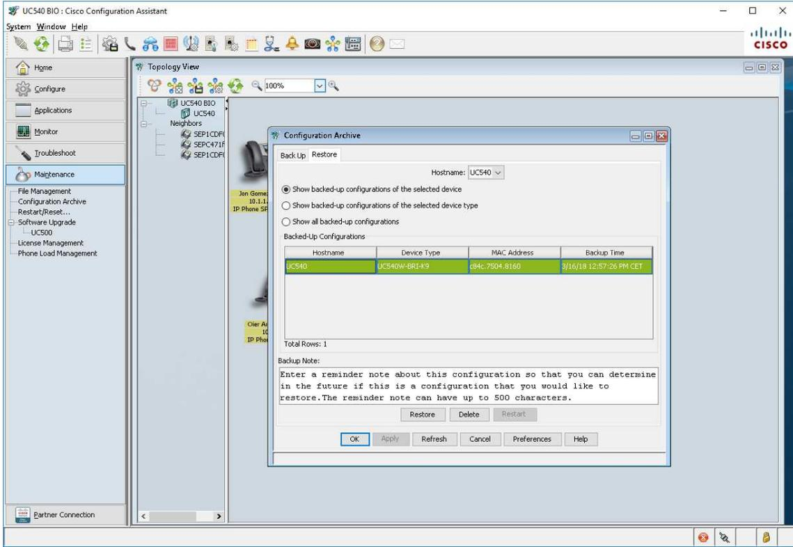
The screenshot shows the Cisco Configuration Assistant interface for a UC540 BIO. A 'Configuration Archive' dialog box is open, displaying a table of backed-up configurations for the selected device (UC540). The table has the following data:
